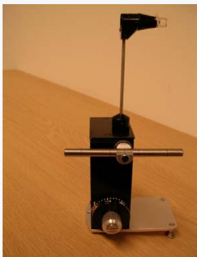
Fig 1a The Goldmann Applanation Tonometer (GAT) is slit lamp mounted and although considered the ‘gold standard’ for tonometry measurements, is not practical for use in a domiciliary setting
